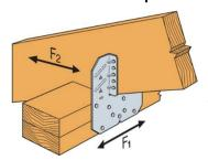
**Strapping/Ties/Hurricane Straps** should be used to connect rafters to the top plate. On open structures or even in wind-uplift events (storms) the wind is trying to force the roof to blow away. These straps will give a structure the extra strength it needs.
